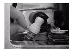
5. Insert the screwdriver blade against the locking ring and pull down on the hose.
